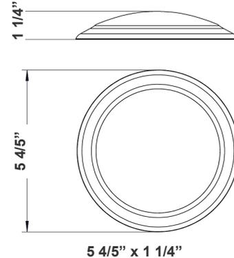
Disk lights have been designed to be a flexible lighting solution for retrofit and new construction applications, Ideal for closets, storage areas, attics, corridors, or general lighting solutions for residential and commercial applications.
