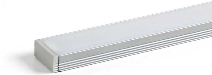
The ALP-20 is an Architectural-grade LED extrusion designed for surface mount applications and can fit linear LED strips up to **12mm (0.5")** wide. Made from high quality aluminum and manufactured with a patented frosted diffuser for maximum lumen output and wider beam distribution.
